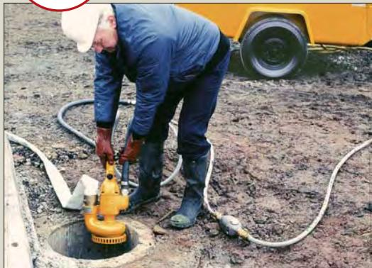
Rugged body construction in cast iron – Simple transfer requiring high flow (750 l/min average) with high discharge head (20 metre average).
